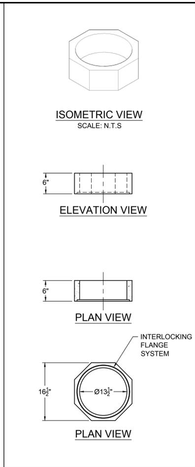
**DM54 FLUE-Ø14" INNER LINER AND Ø14" STARTER BLOCK**
