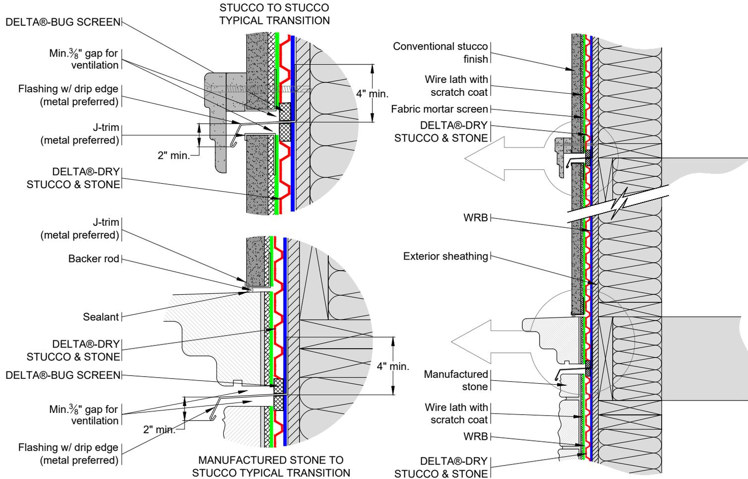
**\*\*For proper performance of DELTA®-DRY ensure top and bottom remain open to allow ventilation and drainage\*\***
