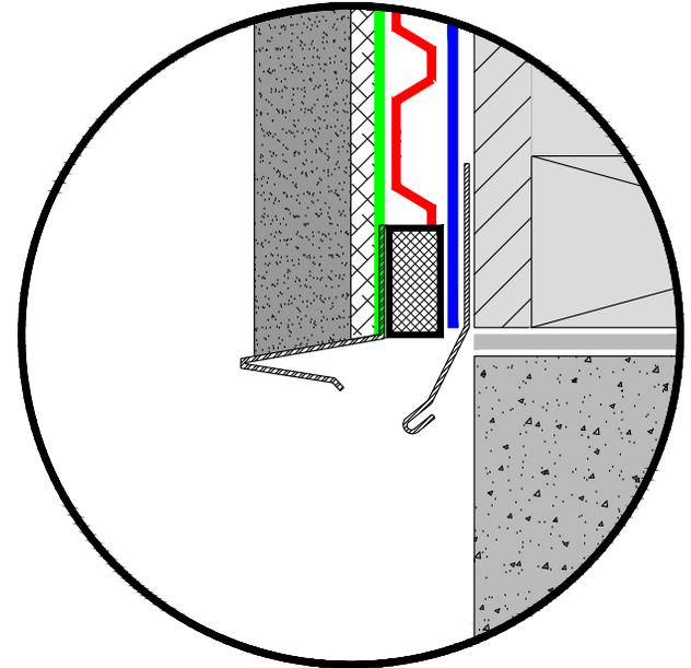
**\*\*For proper performance of DELTA®-DRY ensure top and bottom remain open to allow ventilation and drainage\*\***
