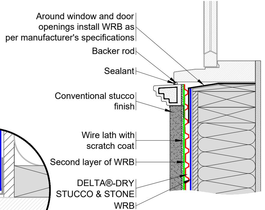
**\*\*For proper performance of DELTA@-DRY ensure top and bottom remain open to allow ventilation and drainage\*\***
