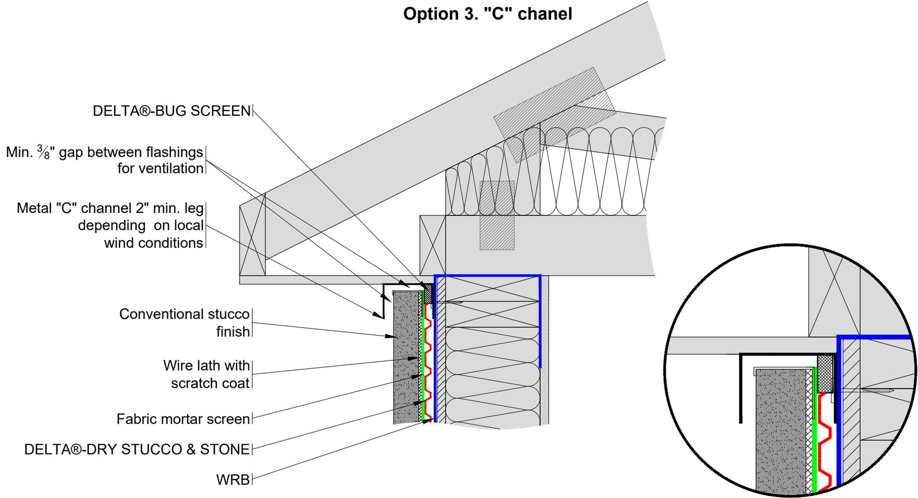
**\*\*For proper performance of DELTA@-DRY ensure top and bottom remain open to allow ventilation and drainage\*\***
