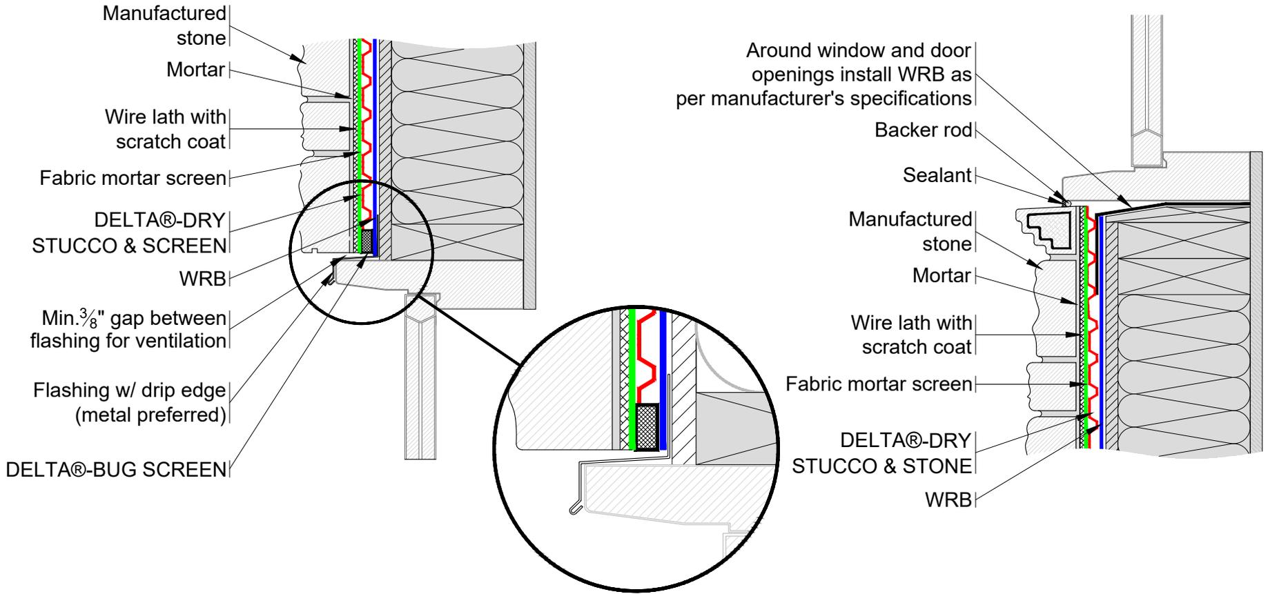
\*\*For proper performance of DELTA®-DRY ensure top and bottom remain open to allow ventilation and drainage\*\*
