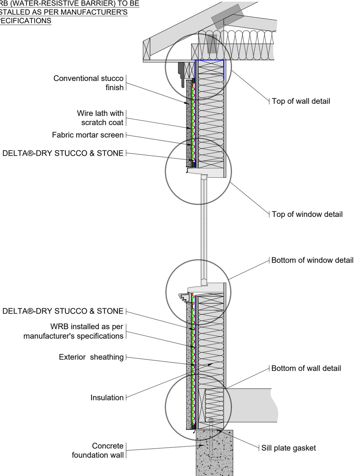
**\*\*For proper performance of DELTA@-DRY ensure top and bottom remain open to allow ventilation and drainage\*\***
