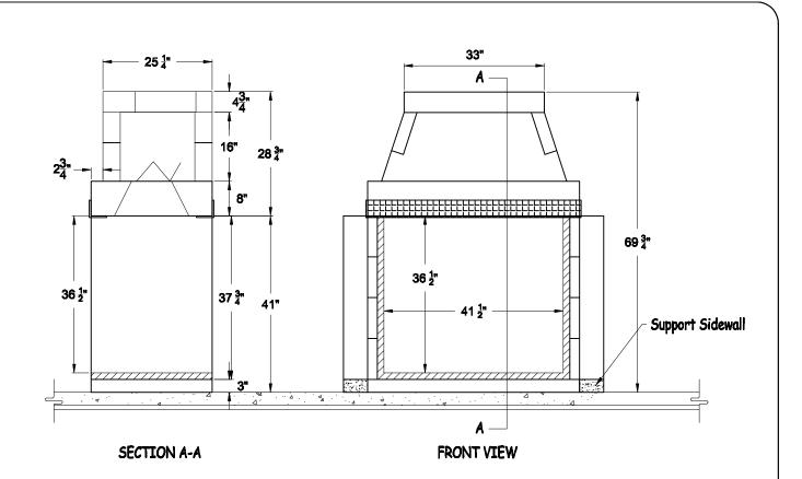
PLAN, SECTION and ELEVATION of ISOKERN 42 SEE-THRU FIREPLACE
