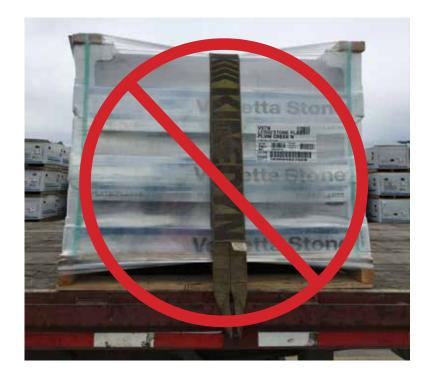
Care must be taken when removing Versetta packages from the trailer. Do not pull the pallets out without first loosening the 2"x4" board. Lift the top pallet straight up to loosen and remove the 2x4's. Take caution with this board once it is loose.
