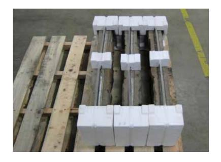
Ensure the product is securely fastened to the pallet. If banding is used do not apply pressure to the nail strip or the product. Do not stack other heavy materials on top of the product.
