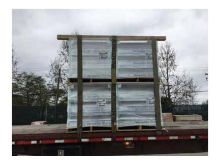
Incorrect orientation of the pallet could result in damage to the product and potential for load to shift during transportation.
