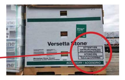
Double stacking of the pallets is acceptable if each pallet is placed directly on top of the pallet below and the previously noted guidelines are followed.
