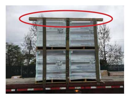
DO NOT position the straps over the center of the package without double 2x4 being secured to the package. Positioning the straps in this location will cause damage to the product and and potential for the load to shift during transportation.
