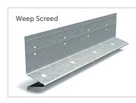
protects these susceptible framing materials. The weep screed also acts to kick the water out from the building and provide the appropriate clearance from grade or a paved surface. In most cases, the weep screed is installed to provide a 4" clearance from grade or a 2" clearance from any paved surface. The weep screed is the first to be installed so that WRB materials can lap over its 3" attachment flange in shingle fashion.
