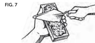
**Note:** In tight fit applications, before placing next unit, compact or remove the squeezed out mortar to allow adjoining unit to butt tightly. There shall be mortar between the units but the joint will be less than 3/8."
